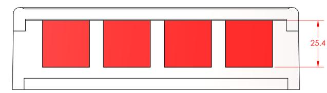
Using #102 DD lid you can put upto 66.6 x 25.4 x 3mm
