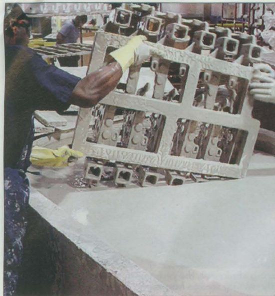
Fig. 1. For many years, the assembly trees were manually dipped into the coating mixture, as seen above, but advances in manufacturing processes have led to the automation of both clustering and dipping.
