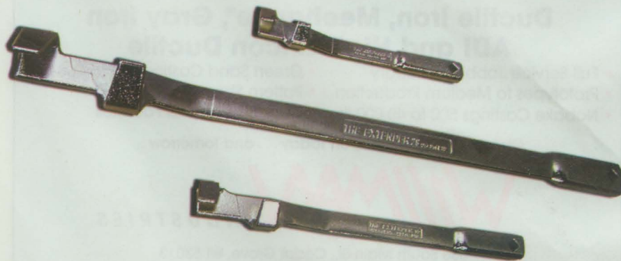
This wrench extender made of manganese-bronze and cast-in via lost foam required no draft between the ears, included a cast hole and required no risers.
