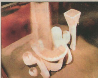
In lost foam casting, the foam pattern is placed in a flask and loose, unbonded sand is poured in and around it, as shown above. Vibrations compact the sand into the internal passageways, and after compaction, molten metal is poured into the mold.
