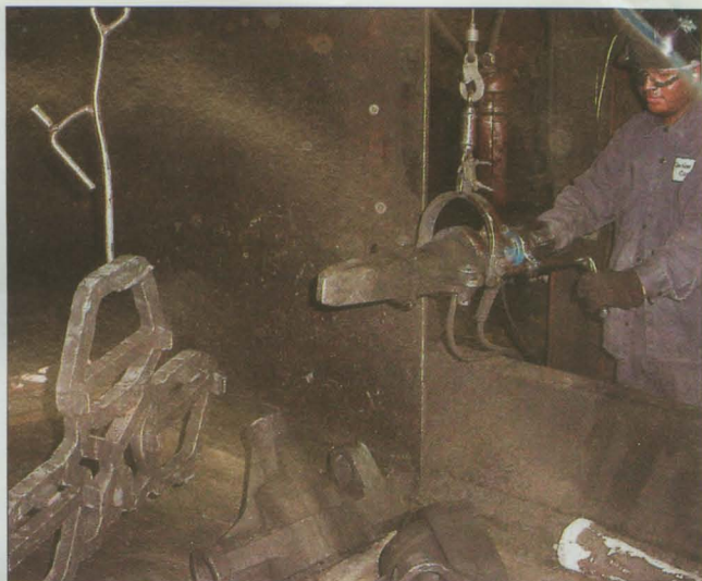
Fig. 3. During shakeout, the pneumatic wedge, which replaced a manually-swung sledge hammer, separates the casting from the runner.
