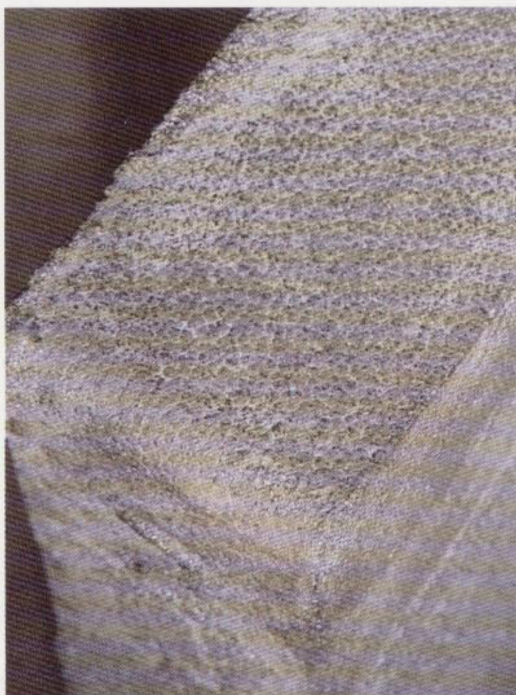
Casting from PMMA pattern
