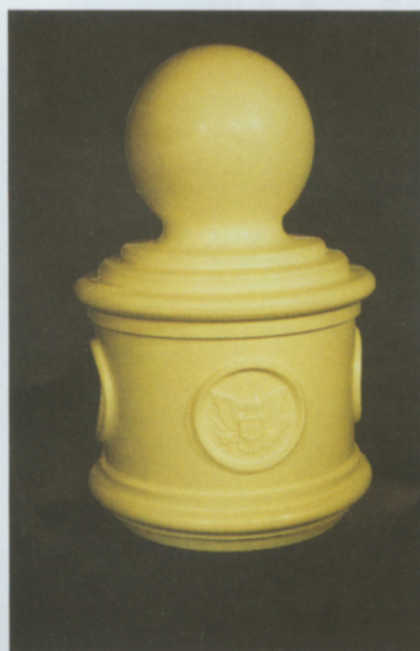
Tempo's foam patterns have been used for complex applications, left. The Bollard Cap for the U.S. Capitol perimeter security, shows good cast detail in the Eagle emblem, right.
